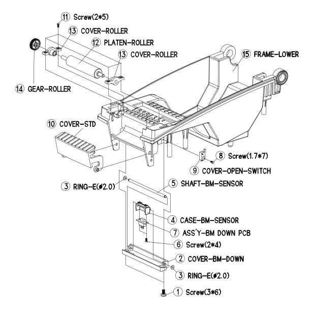
Figure 5-13 Disassembly FRAME-LOWER #4
