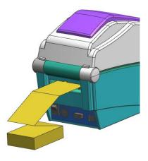
2) Adjust Paper Holders to the paper width by using the Fix Tool.
