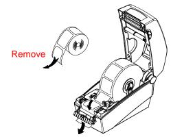
4) Adjust the paper guides and close the label peel-off cover.
