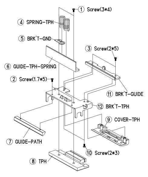
Figure 5-7 Disassembly UPPER #5
