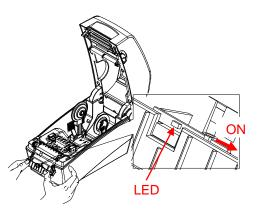
3) Remove one sheet of the label paper, and insert the paper as shown in the image below.
