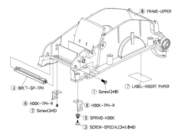
Figure 5-9 Disassembly UPPER #7
