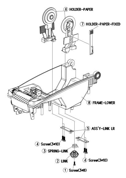
Figure 5-10 Disassembly FRAME-LOWER #1
