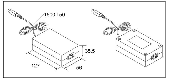
Figure3-2 AC/DC Adapter Dimension
