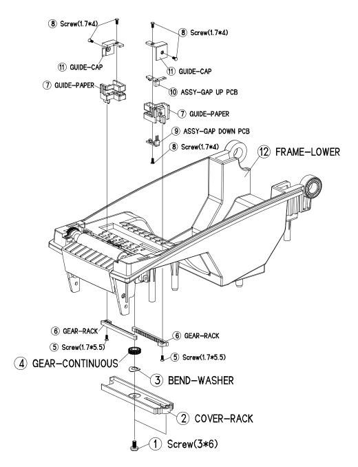
Figure 5-12 Disassembly FRAME-LOWER #3
