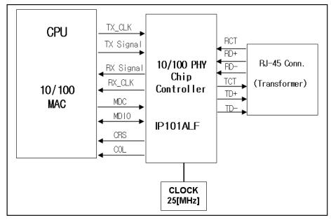
Figure 4-5 Ethernet Communication Block Diagram
