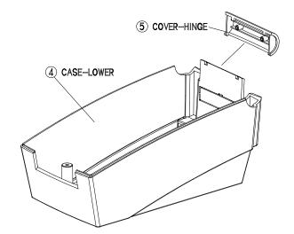
Figure 5-1 Disassembly CASE-LOWER #1
