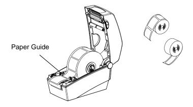
4) After Installation the paper, manually set the sensor (Gap & Black-Mark) and Paper Guide to the correct position.
