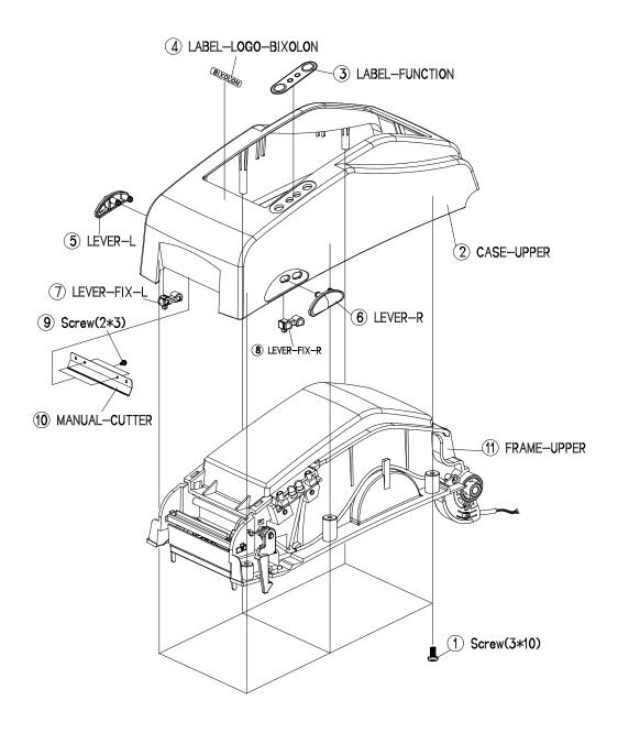
Figure 5-4 Disassembly UPPER #2
