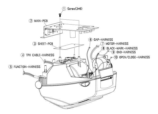
Figure 5-2 Disassembly MAIN-PCB #1
