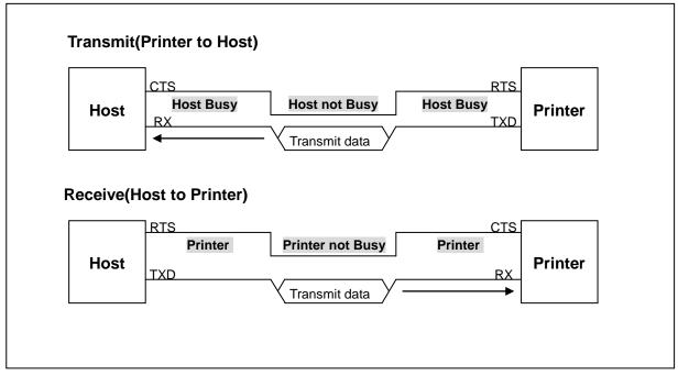
Figure 4-3 RS232C Communication Waveform
