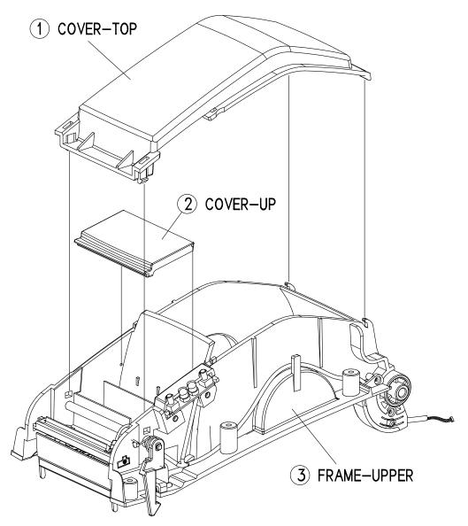
Figure 5-5 Disassembly UPPER #3
