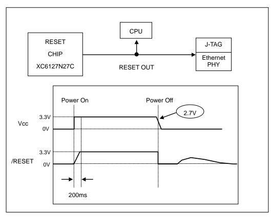
Figure 4-1 Reset Circuit
