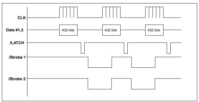
Figure 4-7 Thermal Printer Timing Waveform
