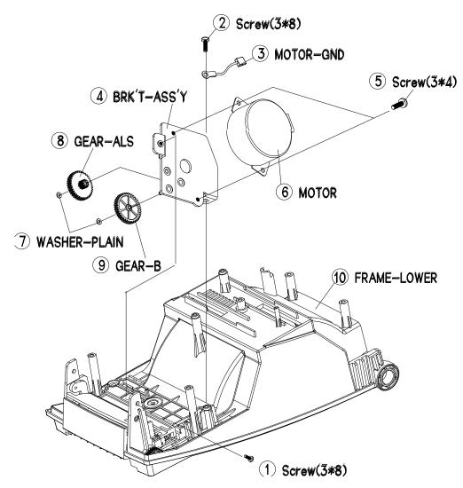
Figure 5-11 Disassembly FRAME-LOWER #2
